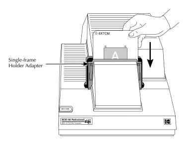
The film holder is now properly inserted into the Scanner.
